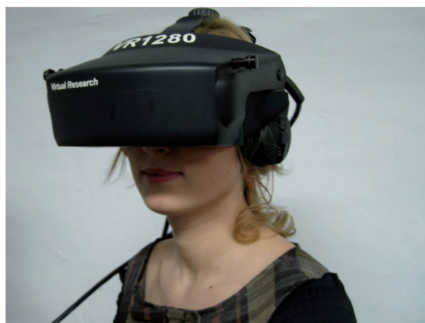
Figure 1 Image of a head mounted display for visualization of 3D virtual environments.
